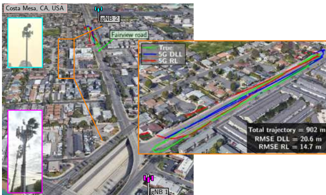
Fig. 6. 5G gNBs' locations and traversed trajectory: true (white), DLL-based estimate (blue), and RL-based estimate (red). Image: Google Earth.
