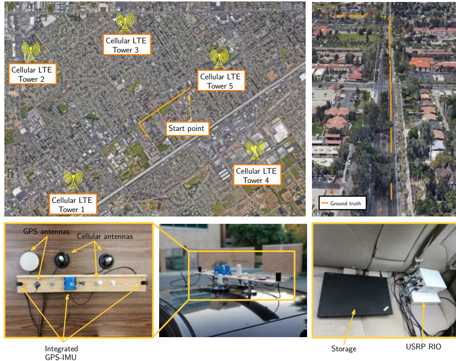
Fig. 2. Experimental hardware setup and the traversed trajectory along with the position of cellular LTE towers. A ground vehicle was equipped with an integrated AsteRx-i V GPS-IMU sensor, cellular antennas, and USRPs. The ground vehicle traveled 1.35 km in an urban area (downtown Riverside, California) collecting GPS, IMU measurements, and cellular LTE signals from five cellular towers.
