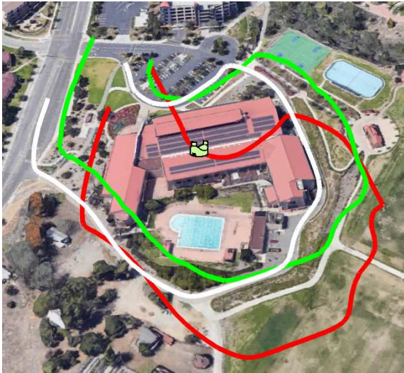
Fig. 9. Receiver trajectory (white) and navigation solutions obtained using the NNDLL (green) and the E-L DLL (red).
